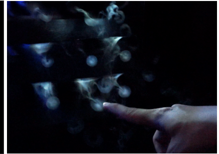
Figure 3: Volumetric pixels in the air.
